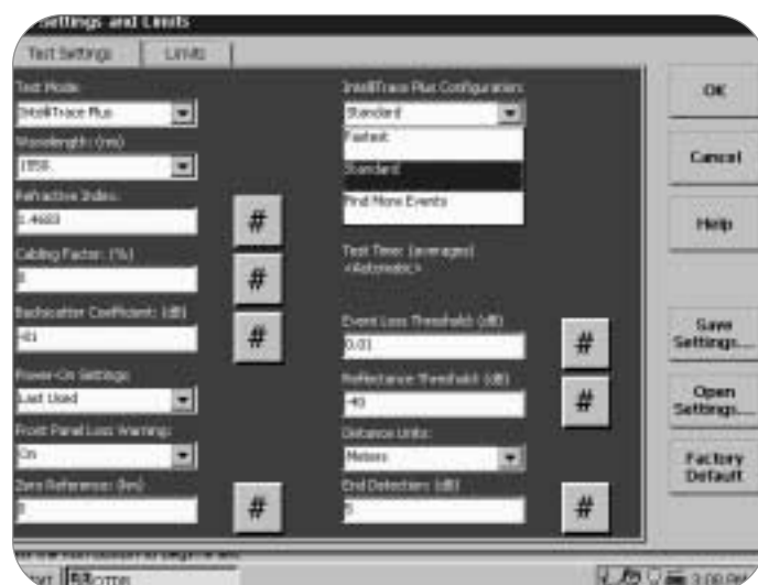
► Figure 2: Screen shot of Settings window with IntelliTrace Plus options drop-down menu open.
